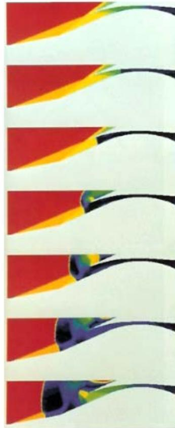
Fig. 6 Visualization of unsteady hypersonic flow; Ramjet unstart. Isofringes for the pressure field.
