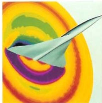
Fig. 4 Pressure field in a cross section generated by the wing-body configuration of a generic supersonic transport aircraft.
