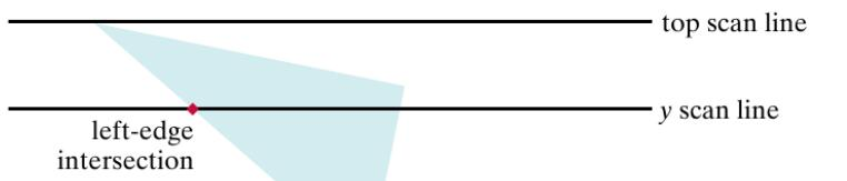
**FIGURE 9-6** Scan lines intersecting a polygon surface.
