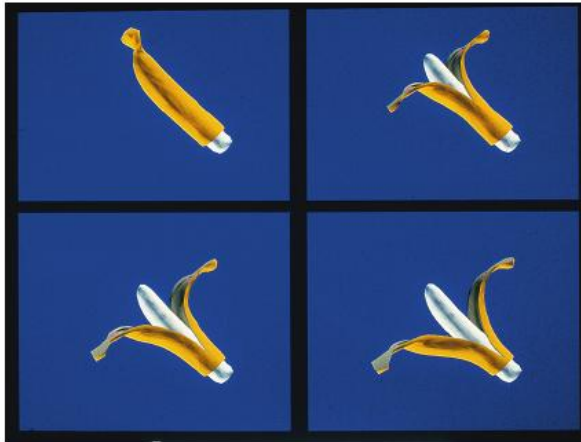
FIGURE 8-120 Modeling the flexible behavior of a banana peel with a spring network. (Courtesy of David Laidlaw, John Snyder, Adam Woodbury, and Alan Barr, Computer Graphics Lab, California Institute of Technology. © 1992.)
