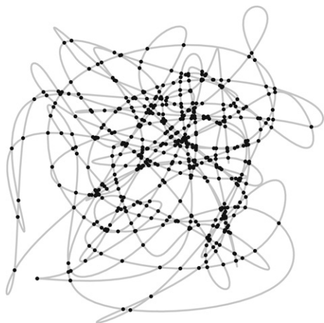
Fig. 9. Several hundred self-intersections of this periodic cubic B -spline curve with one hundred control points are identified in less than a second on a modern PC workstation, using the (u - v) elimination approach.
