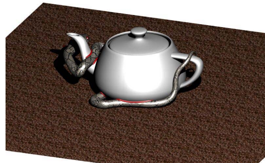
Figure 10. Intersection between the Utah teapot and a ringed surface.
